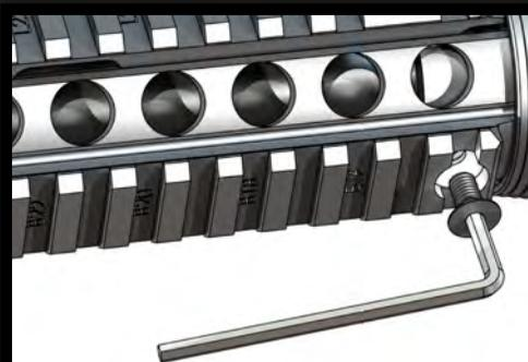
Figure 4 - Installing Screw
